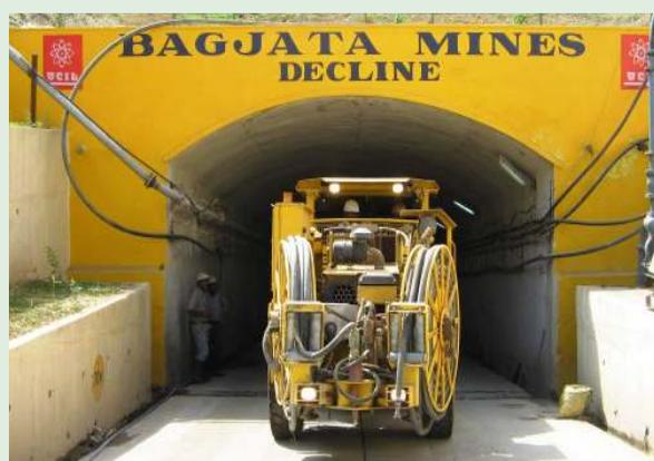
1<sup>st</sup> December 2008. The mine uses trackless equipment like Drill Jumbo, LHDs and LPDTs. The mine is expected to reach its full capacity during 2009-10. A vertical shaft upto a depth of 375m has been sunk. Head frame erection and equipping are expected to be completed by 2010-11.
